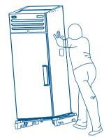
A Incline the equipment, locate the screws and remove them with a screwdriver.
