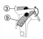
FIG 4. UNLOCKING THE GRIP
